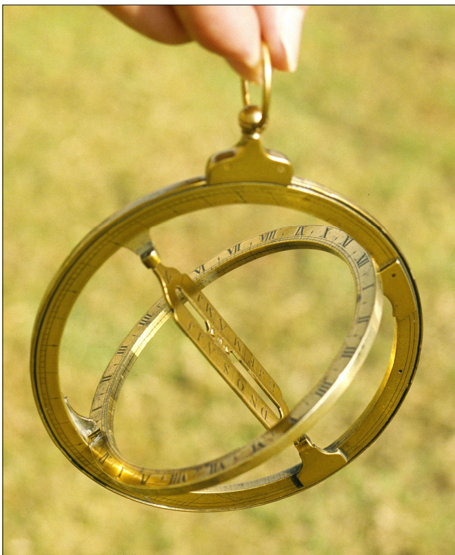
Fig. 11. An 18 th century universal equinoctial ring-dial, in use.
