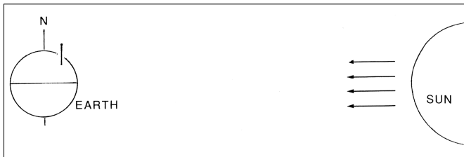
Fig. 9. Sun-Earth geometry for sun's declination of zero.
