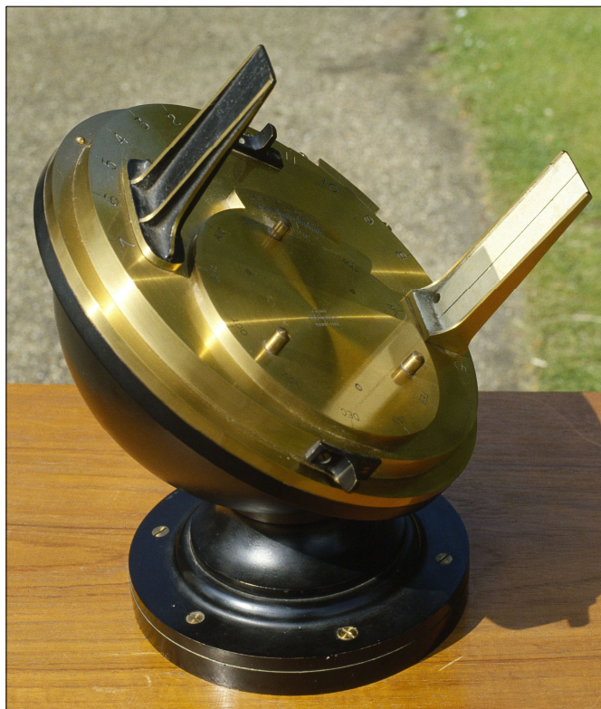
Fig. 16. The famous Pilkington & Gibbs heliochronometer, patented in 1906 and exported widely around the world.
